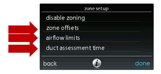
Zone Offsets allows adjustment of zone temperature sensors +/- 5 degrees.
