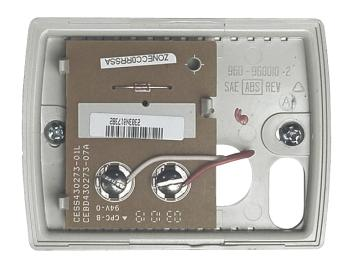
If sensor is wired to ZS1 on the damper control module or S1/S2 on the UI, then this will override the temperature sensed by the UI.
