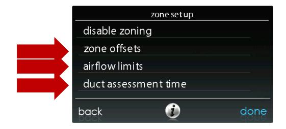
Zone Offsets allows adjustment of zone temperature sensors +/- 5 degrees.
