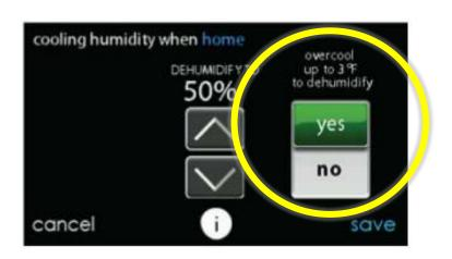
Note: When turned on the system will allow a 3-degree overcool for dehumidification. Will never overcool-to-dehumidify below 70-degrees.
